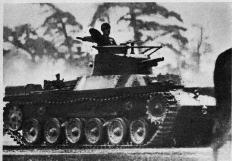
Jap medium tank 2597 head-on looks like U. S. General Grant with off-center turret. Gun shown is a low-velocity 57-mm. Hull is long, narrow and low. Light track (see below) has six medium bogie wheels.
